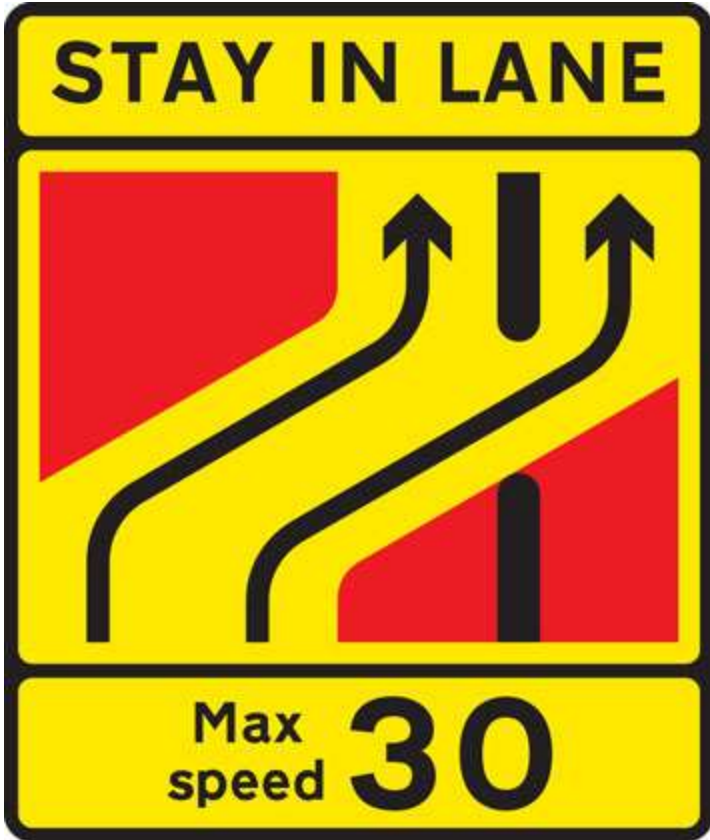
One lane crossover at contraflow road works
