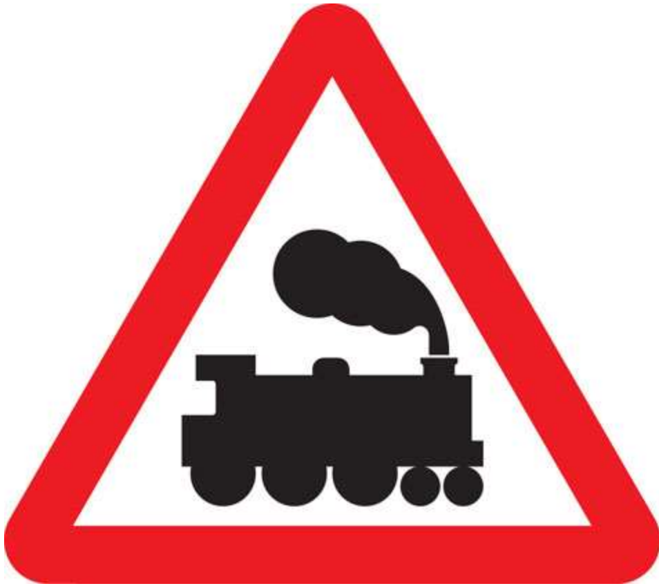
Level crossing without barrier or gate ahead
