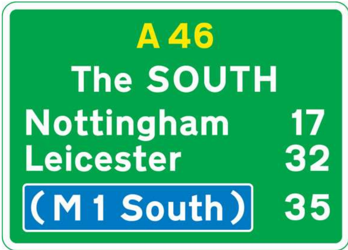
Route confirmatory sign after junction
